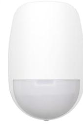
DS-PDD12P-EG2-WB is a fully supervised two-way wireless detector featuring motion and microwave detection, tamper protection, low battery and supervision. It can operate for up to 5 years from two in-built batteries, and monitors the area within 12m radius, ignores animals while recognizing human from the first step.
