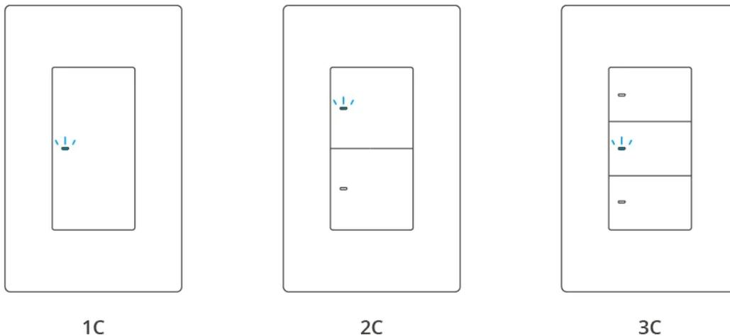
ⓘ The device will exit the pairing mode if you do not operate it within 3mins. When you want to enter the pairing mode again, long press the any button on the device for 5 seconds until the signal light “flashes slowly” and release.
