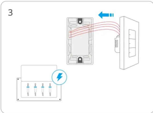
Install the device into the mounting box first, then power it on.
