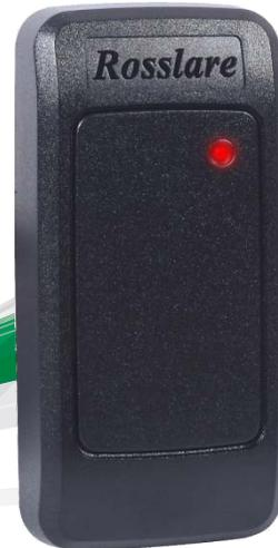
ROSSLARE'S AY-K12 IS A POWERFUL RFID PROXIMITY CARD READER OF 125 KHZ CARDS AND TAGS, FEATURING WIEGAND 26-BIT OUTPUT FORMAT AND A READ RANGE OF UP TO 3.15 IN. (80 MM).
